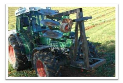
Figure 2-6 Cutting the grassing (seeded + spontaneous), and triturating of foliage pruning, with decentered hammer-type blades machine
