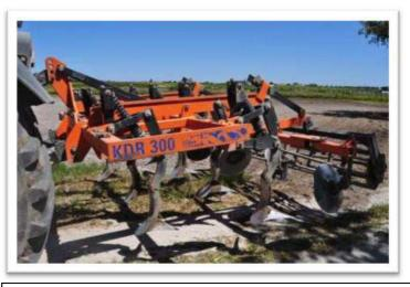
Figure 2 2Combined machine of spring-loaded tines with straw incorporated discs to prepare the soil with fewer passes and less fuel and energy consumption
