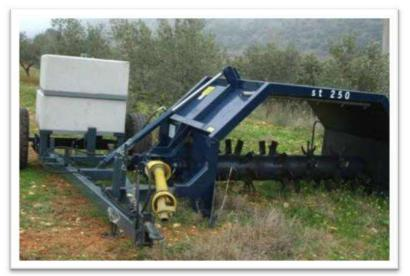
Figure 2 9 Equipment for turning and aerating compost
